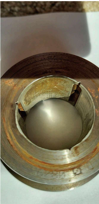
Figure 2. Varnish deposits on a bearing. Figure courtesy of Daryl Beatty.
