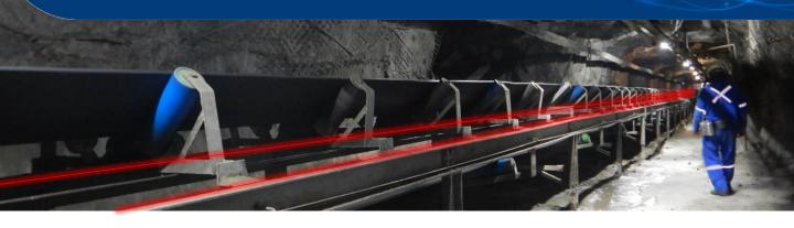
The **LUNA EX.TRACT** system transmits laser pulses through a retrofitted fibre optic cable along the conveyor system.
