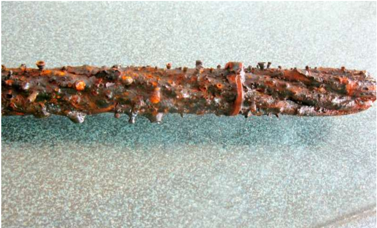
Green cable tie – CorrosionX Heavy duty sample after 1000 Hrs NSS.
