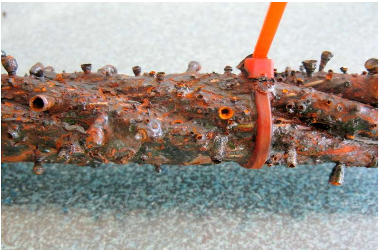
Red cable tie – reference sample after 500 Hrs NSS.
