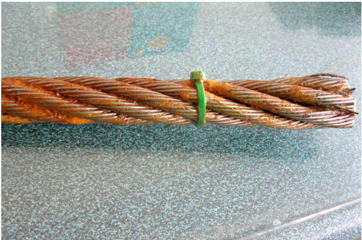
Green cable tie – CorrosionX Heavy duty sample after 1000 Hrs NSS.
