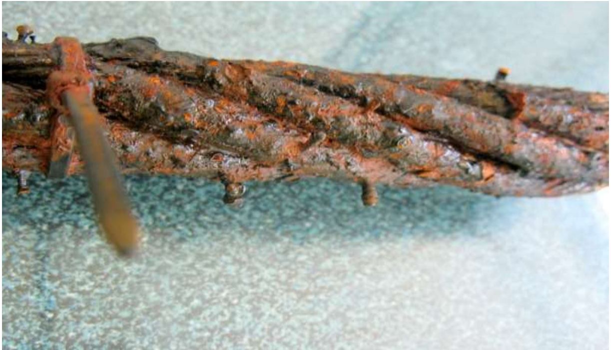
Black cable tie – Imported wire sample after 500 Hrs NSS
