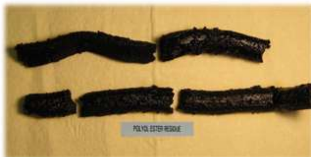
Figure 4. Polyol ester gels from an aluminum plant.
