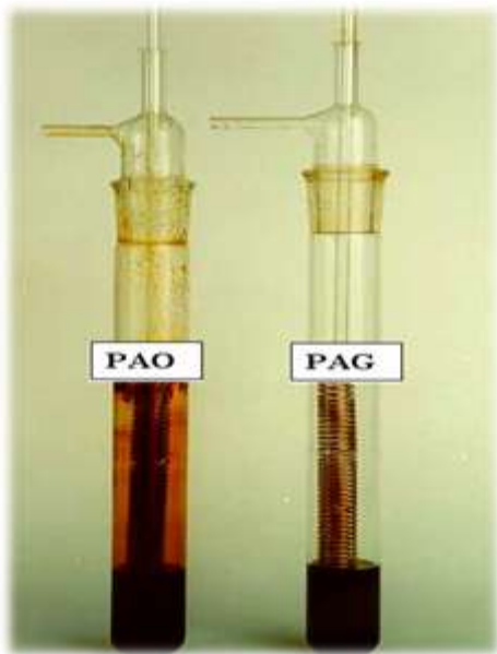
Figure 5. Varnish formed during TOST testing.
